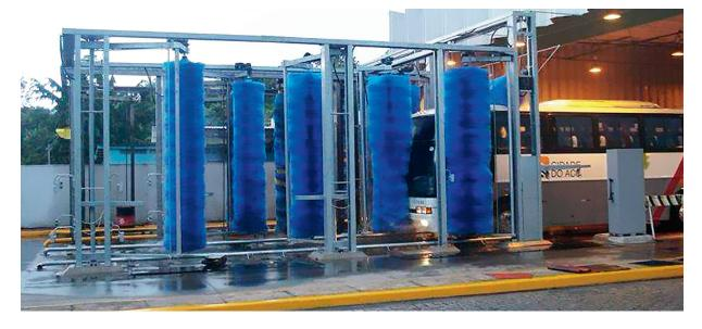
The range includes various washing heights and number of brushes and accessories depending on needs and request. LFO can be adapted to all transport vehicles, including trams or vehicles provided with pantograph.
